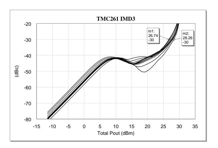
\*VD1 = VD2 = 18V, ID1 = 54mA, ID2 = 20mA, Tamb = 25C, Tone Spacing = 100 MHz
