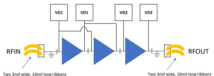
Bias Sequencing: To turn ON the device, VG1, and VG2 are first set at -6V. Then set VD1 and VD2 to 18V. Finally, adjust VG1 and VG2 to achieve ID1 = 54mA and ID2 = 20mA. To turn OFF the device, you set VG1 and VG2 to -6V, then turn off the VD1 and VD2 followed by turning off VG1 and VG2.
