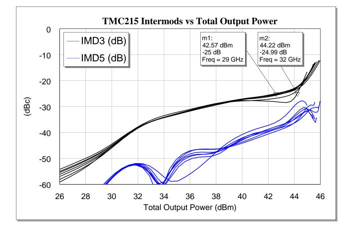
\*VD1 = VD2 = VD3 = 28V, ID\_total = 3000mA, Tamb = 25C Tone Spacing = 100 MHz
