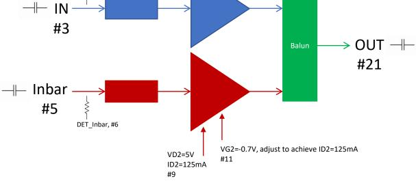
**Bias Sequencing:** To turn ON the device, VG1, and VG2 are first set at -1V. Then set VD1 and VD2 to 5V. Finally, adjust VG1 and VG2 to achieve ID1=ID2=125mA. To turn OFF the device, you set VG1 and VG2 to -1V, then turn off the VD1 and VD2 followed by turning off VG1 and VG2.
