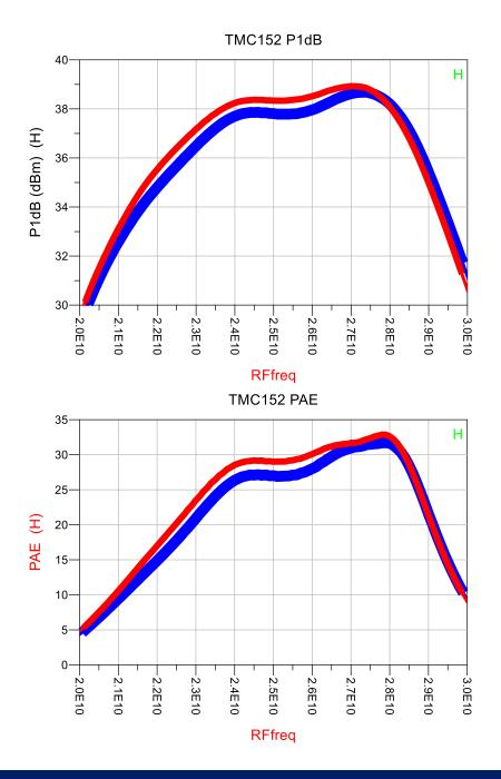
Blue Trace shows the performance at 80 C vs the red trace at 25 C
