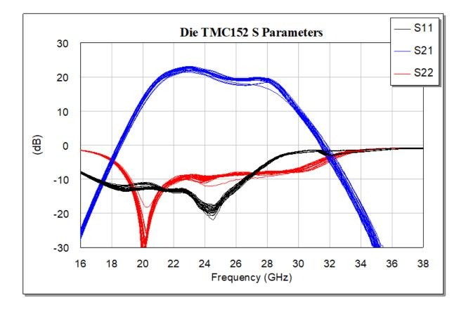
Packaged (TMC152) Electrical Performance on the PCB: Ta = 25 °C, 23V/450mA. measured including PCB transition and Connector Losses
